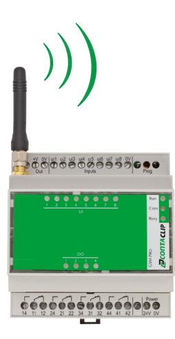
The **GSM-PRO** module features eight multi-function inputs. The input module may be selected as either digital (24 V DC) or analogue (0 to 10V), so that many different signal levels can be connected.
